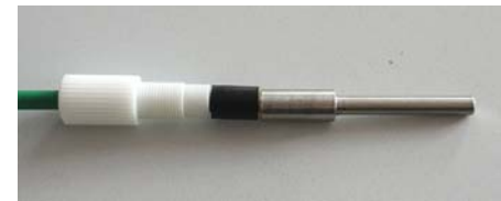
Putting on stainless turning piece
