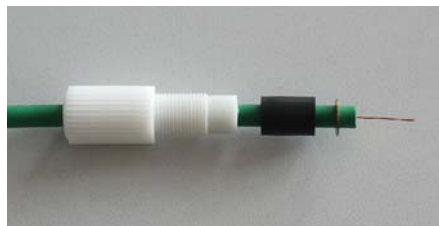
Placing brass washer (Ø10x2 - 0.6mm)
