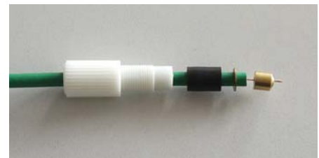
placing brass turning piece (ca. Ø8x8.5mm, tip with cone)
