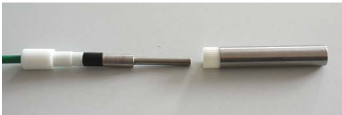
Putting on the probe housing and screwing it with the upper part
