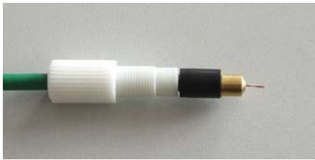
Placing brass turning piece up till cable coating
