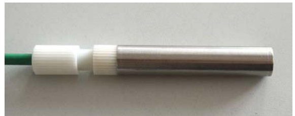
Putting on stainless turning piece
