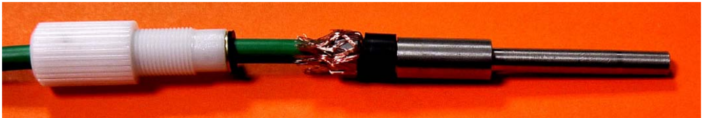
Putting on the stainless steel turning piece
