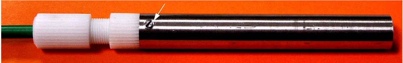
Screwing the threaded upper part of the probe into the housing and fixing the contact screw
