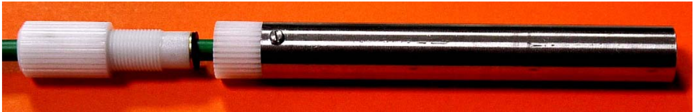
Inserting the cable with the components in the probe housing
