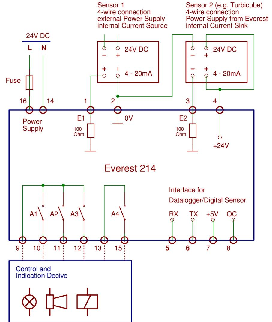
**Sample schematic for sensors with 2, 3 or 4-wire connection**
