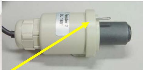
Observe positioning of hole and pin!
