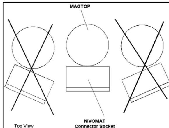
Attaching the NIVOMAT FSG... with Aluminium top to the MAGTOP...
