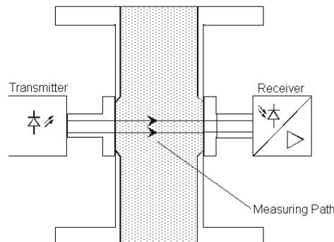
Pulsed infrared light is passed through the liquid medium from the transmitter to the receiver. If the selected turbidity value is exceeded or fallen short of, the output relay in the switching amplifier is triggered.
