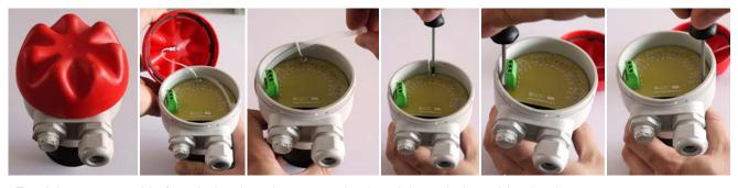
2. Feed the sensor cable from below into the connection head through the cable gland
