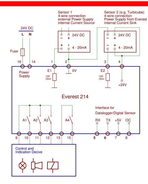
Sample schematic for sensors with 2, 3 or 4-wire connection
