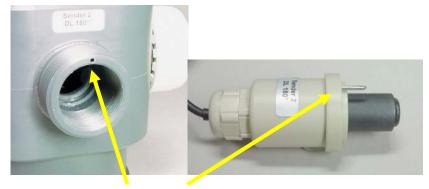
Observe positioning of hole and pin!
