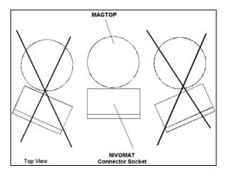
Attaching the NIVOMAT FSG... with Aluminium top to the MAGTOP...
