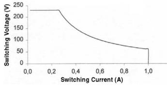
When inductive direct current loads are switched, e.g. with mechanical contractors or relays, increased breaking currents occur which result in interference such as welding of the contacts. For this reason, so-called freewheeling diodes must always be used in such cases.
