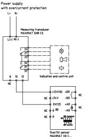
MAXIMAT VK C... to MAXIMAT SHR CS measuring transducer
