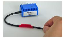
To perform the reset, lift the magnet, which is integrated in the cable and marked with a red shrink sleeving, onto the sticker with the inscription "MÄGNET RESET".
