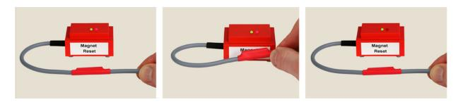
To reset the device, hold the magnet integrated in the cable and marked with a red shrink sleeve against the sticker labelled 'MAGNET RESET'.
