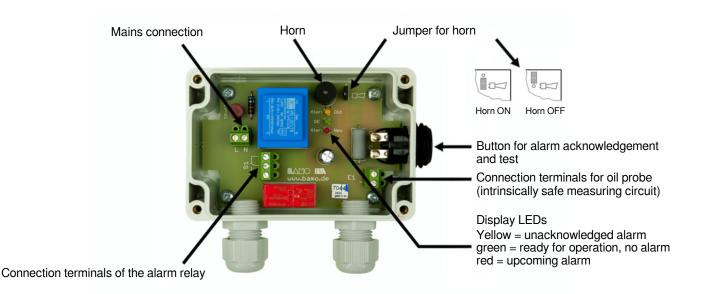
A multi-core cable (5 wires) is recommended for the mains connection and connection of the alarm relay terminals
