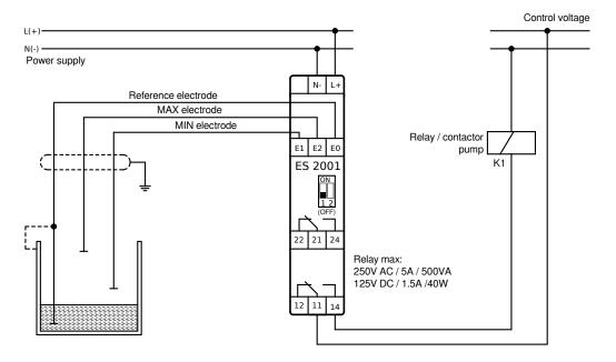
Relay of the filling pump activates when MIN-electrode becomes free; ...drops off when MAX electrode is immersed
