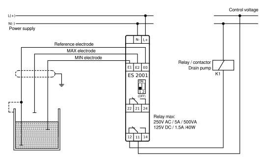
Relay of the drain pump activates when MAX electrode immerses; ...drops off when MIN electrode becomes free
