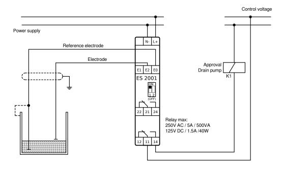
Drain pump relay drops out when the electrode (E2) becomes free or in the event of a fault/power failure/cable break in the electrode control unit
