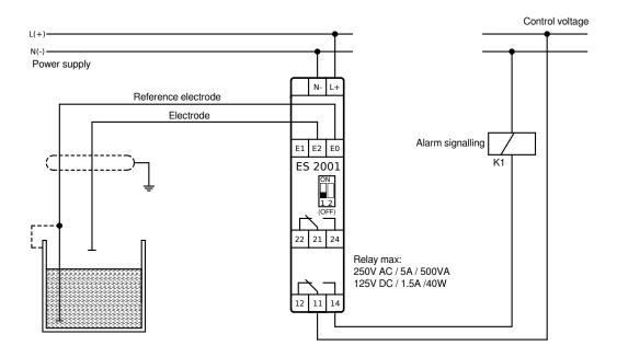
The overfill alarm relay drops out when the electrode (E2) is immersed or in the event of a fault/power failure in the electrode control unit
