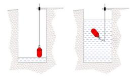
The NIVOSTOP SG2 with a built-in counterweight is mounted freely suspended to its cable. When the liquid level rises or falls, the orientation of the float changes. The mass of the counterweight prevents the float from surfacing.
