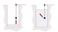
The NIVOSTOP SS2 is a float switch for level control in tanks and catch basins. The cigar-shaped version is designed for introduction in a tank through a small hole of Ø 30 mm.
