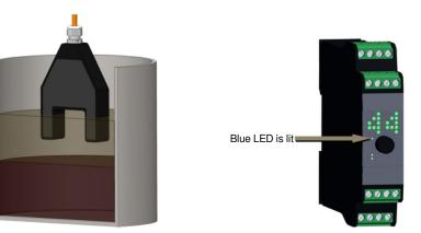
CAUTION: When changing the measuring range (from HIGH to MEDIUM, from MEDIUM to LOW), the blue LED lights up a short time and the relay switches - this only indicates that the measuring range has changed. Depending on the sludge settlement and immersion distance, a switching point could be found in each measuring range (LOW / MEDIUM / HIGH).
